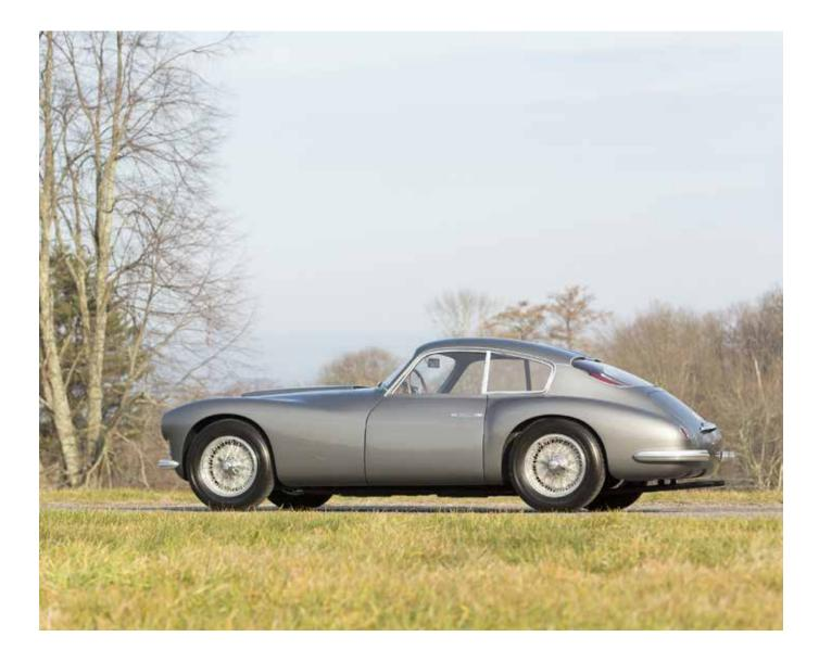
independent suspension (a Fiat first), and Borrani wire wheels with Rudge knock-off hubs. Completed chassis were sent to the Carrozzerie Speciali FIAT in Lingotto, where they were clothed with an elegant new coupe design by Fabio Lucio Rapi that was aerodynamically finetuned in the Turin wind tunnel. The Otto Vu made its public debut at the Geneva Salon in March 1952, and immediately impressed all who saw it with Fiat's ability to produce such a jewel-like automobile.
